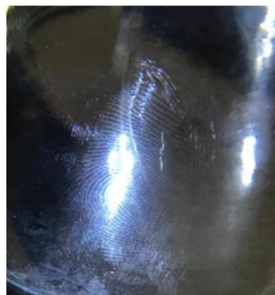
Fig. 9. Developed fingerprint on glass surface
