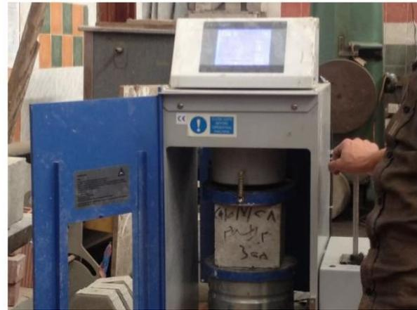
Fig. 2. Concrete cubes testing
