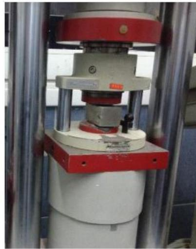
Fig. 6. Compressive strength test of grout prism
