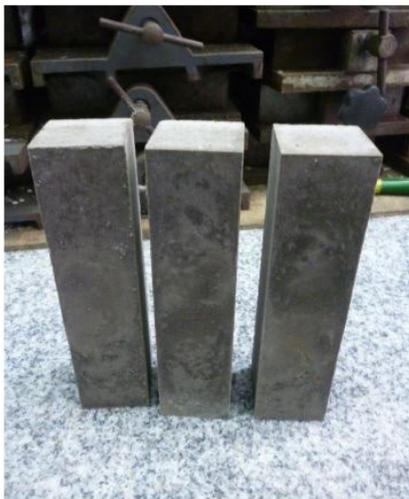
Fig. 5. Grout prisms
