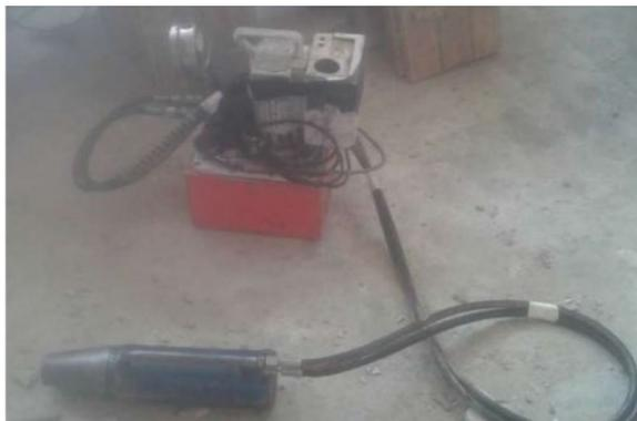
Fig. 9. The jack using for tensioning tendons
