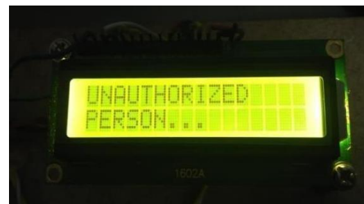
Fig. 12. Display showing about an unauthorized person tries to play the movie
