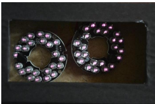
Fig. 10. IR LEDs being turned on
