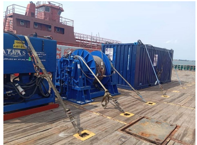
Fig. 4. Cargos lashed to the PSV deck using lashing belts
