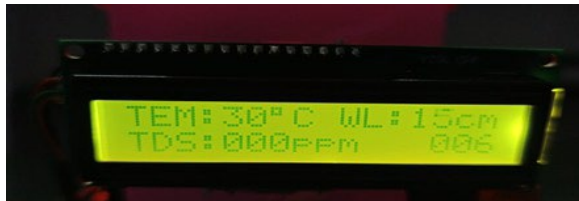
Fig. 7. Output showing temperature, water level and TDS of water
